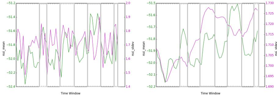
**Figure 5.3:** Bellyband RSSI data over time before application of a Kalman filter (left), and after (right), with mean and standard deviation plotted over 8-second time horizons. The RSSI mean can be more easily observed after filtering from the actuating (highlighted in boxes) and non-actuating time windows.
