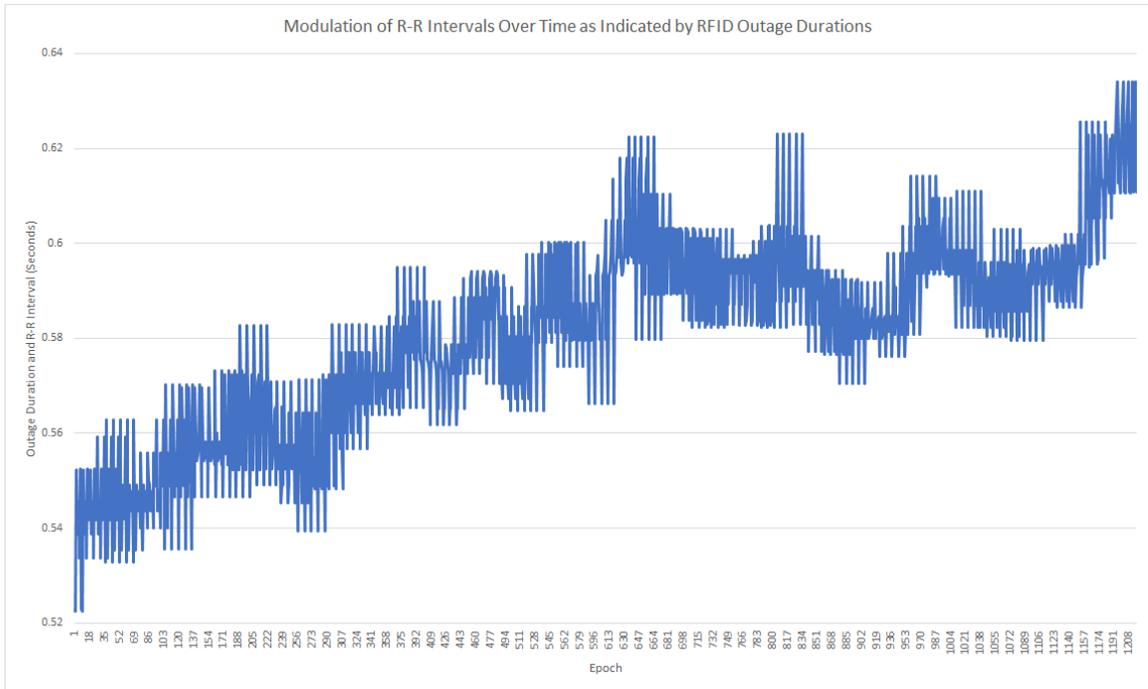
**Figure 13.2:** An example modulation of R-R intervals as inferred from RFID outages during heart monitoring over a 145 second period, correlating to respiratory activity
