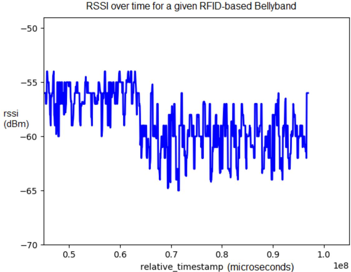
**Figure 12.3:** Sample respiratory data from a programmable mannequin indicating a sudden ambient movement after 60 seconds
