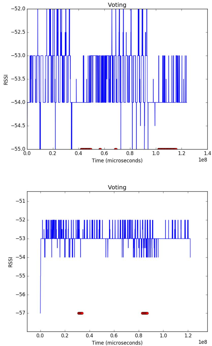
**Figure 12.7:** Classification using voting on multiple MCMC simulator measurements for a human trial at a respiratory rate of 20 per minute (top) and 30 per minute (bottom) with brief cessations: cessation periods are classified along the bottom of the plot
