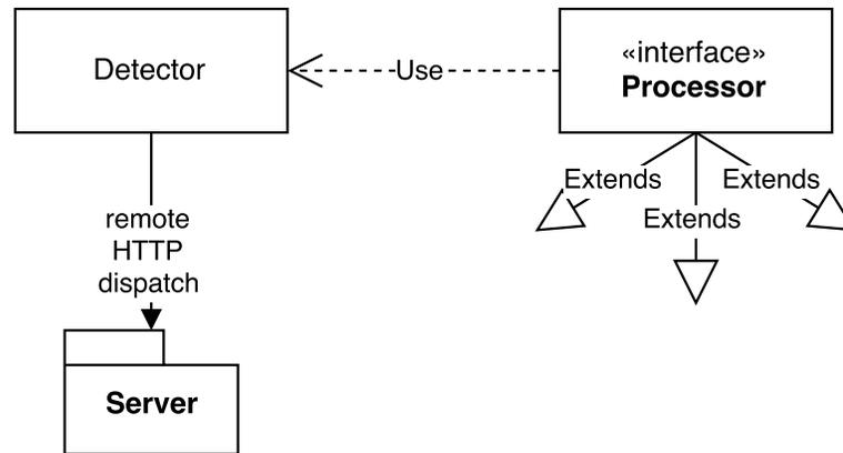
**Figure 6.3:** Modular implementation of signal processing software that utilizes the web service layer to obtain live RFID interrogation data in real-time; here, the **Processor** is a generic interface that is implemented (“extended”) by numerous implementation-specific processors, such as the Short Time Fourier Transform (STFT)
