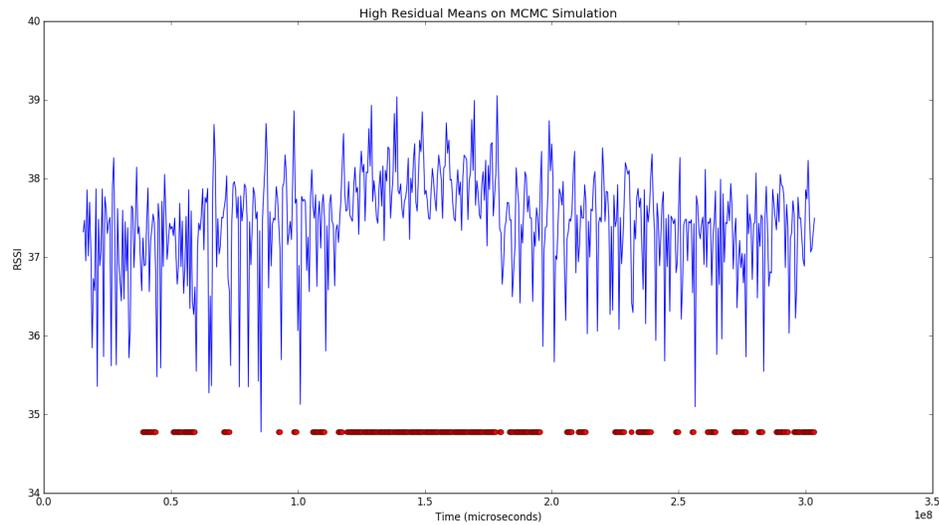
**Figure 6.8:** Retraining conditions are indicated in red along the X-axis of the mean of the residual distribution after removing noise by an MCMC simulation
