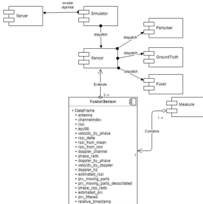
**Figure 9.2:** An architecture diagram of the Fusion Framework that interfaces with the secure data collection and interrogator driver module and respiratory rate measure fusion algorithm modules
