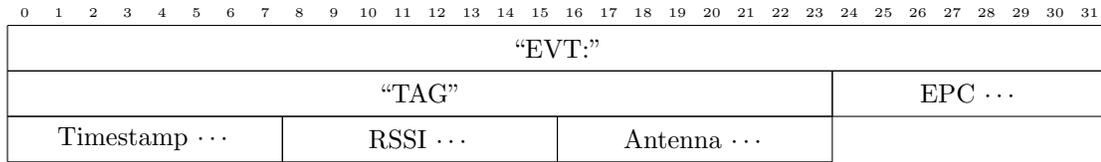
**Figure 4.12:** Bit-level description of an RFID event message sent by the Bluetooth IP30 portable interrogator
