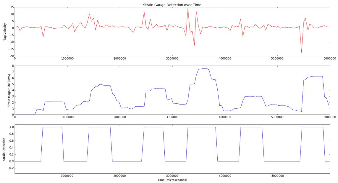
**Figure 8.1:** Correlating the tag velocity and signal strength (top) to form a binary classifier of strain gauge motion artifacts (bottom) by locating the inflection points of a rolling RMS measure (middle) against  $\delta$
