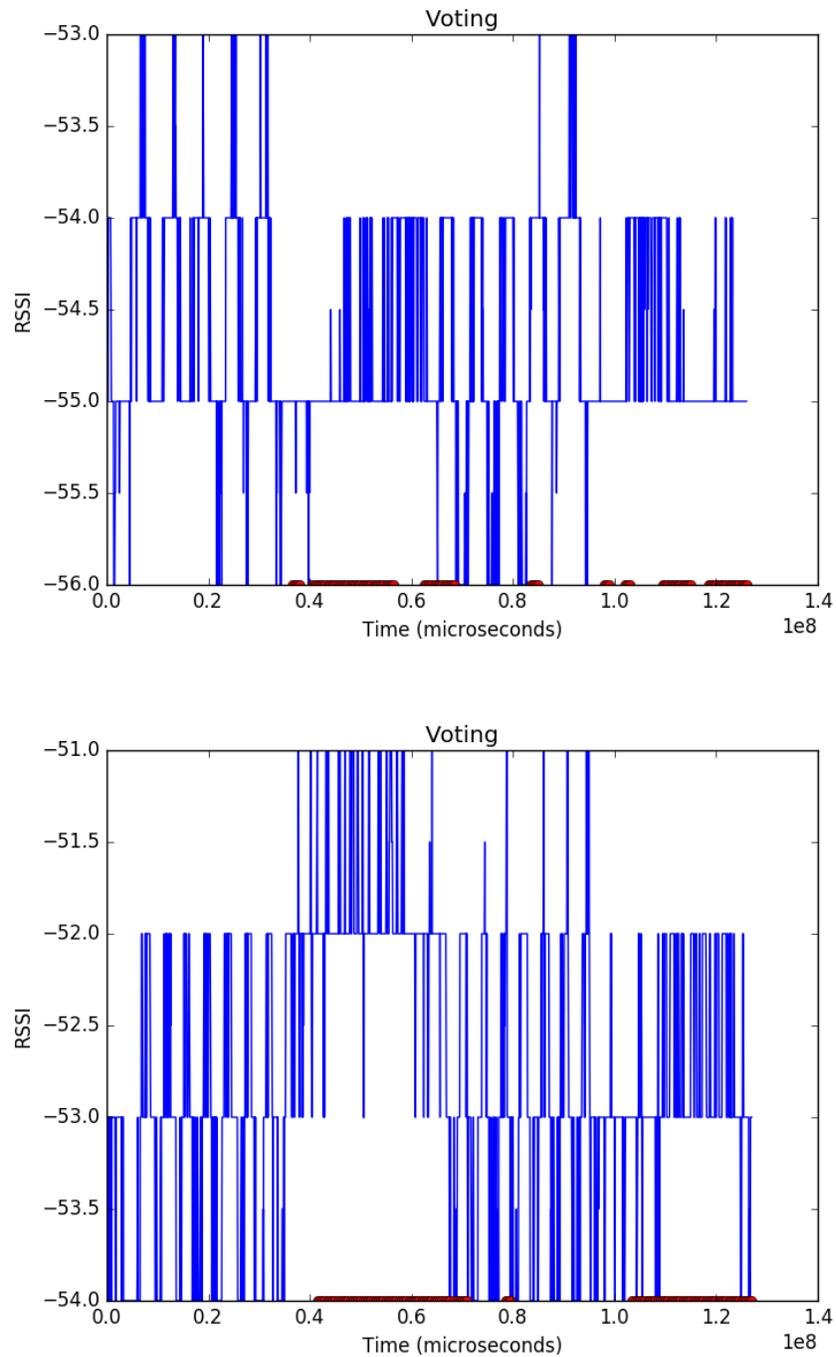
**Figure 12.6:** Classification using voting on multiple MCMC simulator measurements for a human trial at a respiratory rate of 10 per minute (top) and 15 per minute (bottom) with brief cessations: cessation periods are classified along the bottom of the plot
