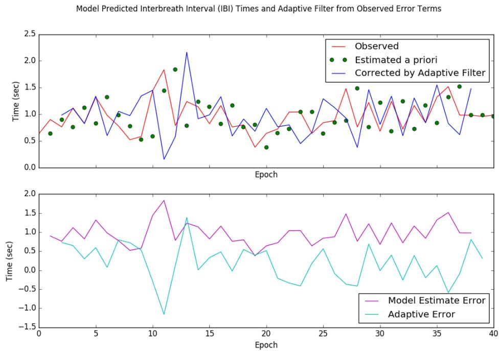
**Figure 10.2:** Convergence of adaptive filtering algorithm using an autoregressive model of probabilistically estimated IBI according to a log-normal historical distribution
