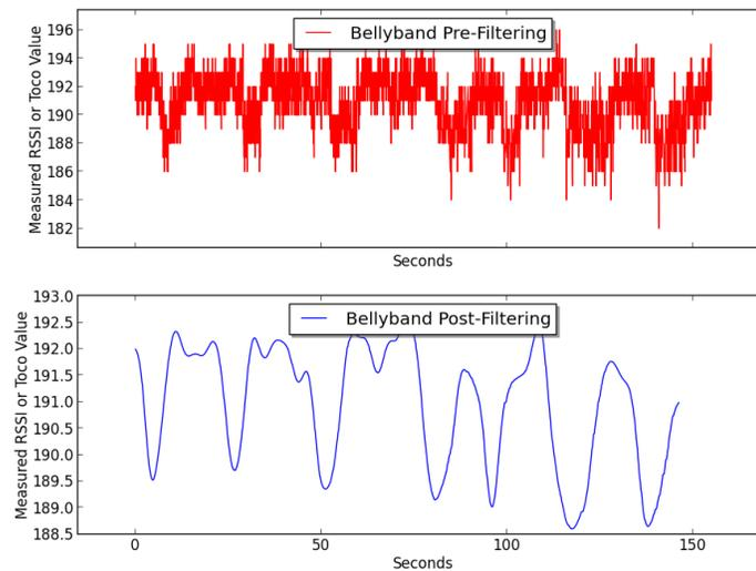
**Figure 6.2:** The raw data (top) collected from the RFID interrogator shows quantization and noise removed by applying a Gaussian filter (below).
