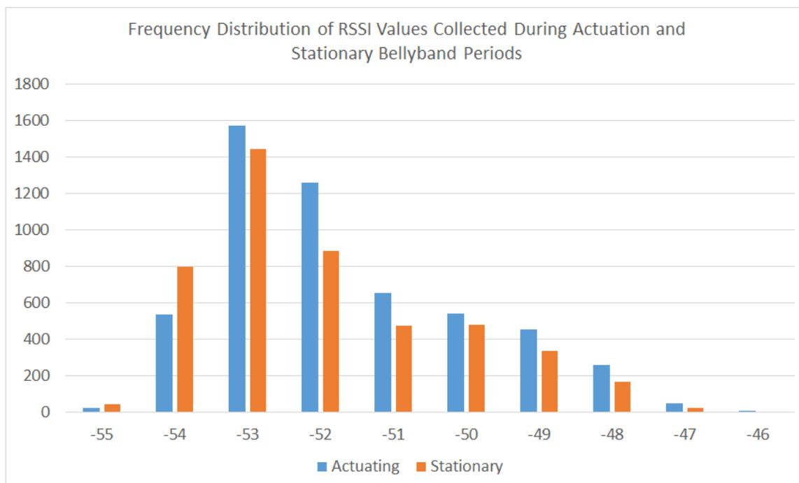
**Figure 6.1:** Histogram of RSSI values collected and separated into actuating “breathing” (left) and stationary “non-breathing” (right) classes, showing the high degree of overlap between the classes
