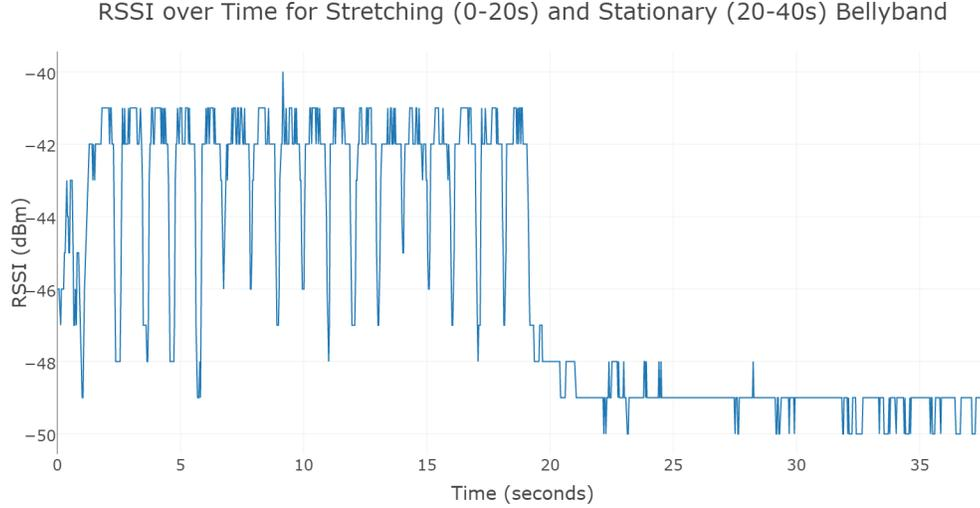
**Figure 1.2:** RSSI time-series data plotted over time for approximately 40 seconds; although oscillatory motions can be observed every second, smaller perturbations in the data obscure this signal due to the RFID interrogation frequency changing every 200 milliseconds
