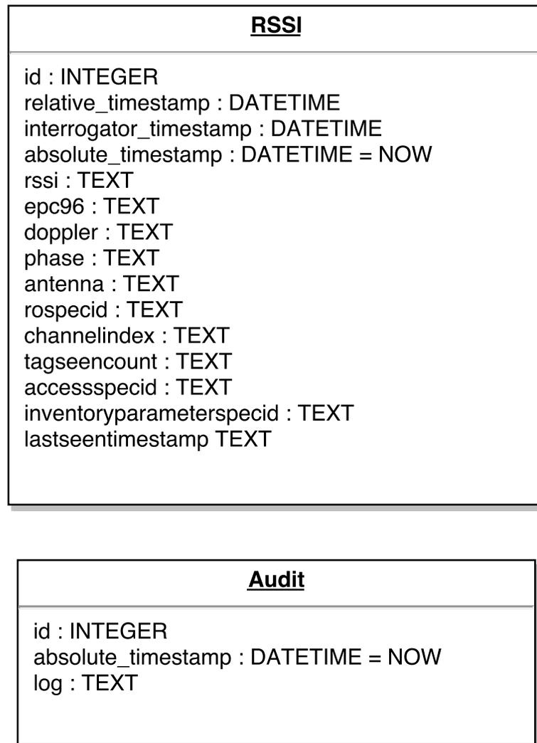
**Figure 4.4:** Database schema for the encrypted RFID data and HIPAA audit table
