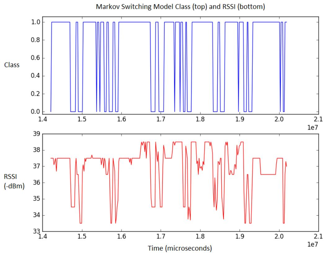
**Figure 6.7:** Result of a Markov Switching Model applied to RFID data for unsupervised classification of wearer state
