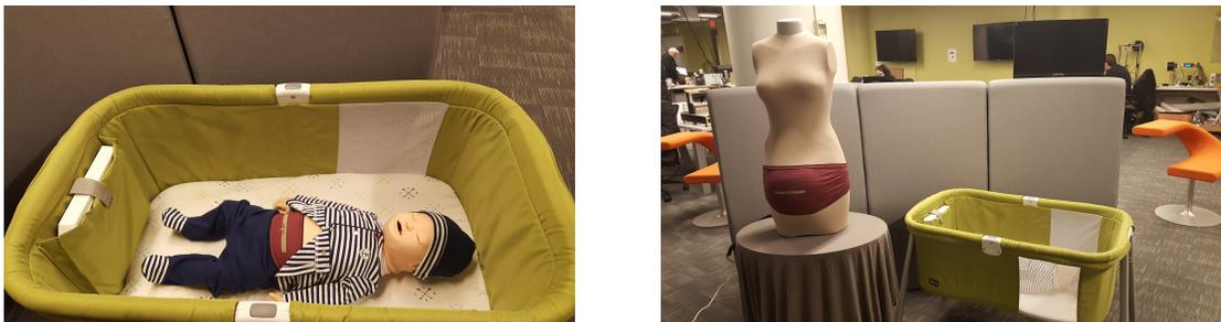
**Figure 1.3:** The knitted smart-garment device Bellyband uses an embedded RFID tag and knit metallic thread antenna to monitor strain-gauge movements such as respiration (left) or a uterine contraction (right).
