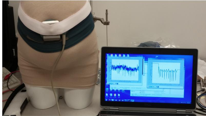
**Figure 4.1:** A tocodynamometer pressure sensor is placed above a Bellyband on a “pregnant mannequin” and monitored using our software (the RFID data plot is to the left, and the tocodynamometer data plot is to the right).
