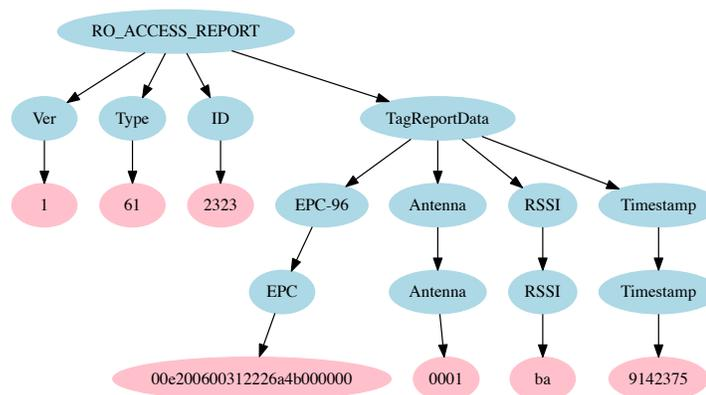
**Figure 4.6:** Structure of a Sample Read Event Message XML Document
