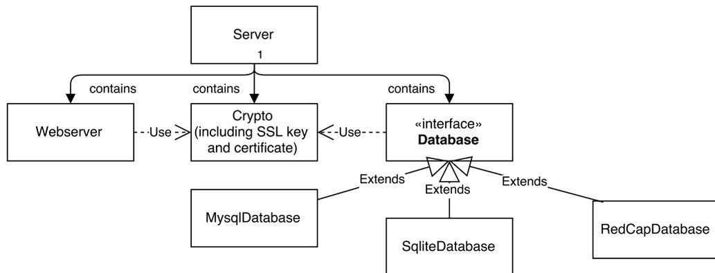
**Figure 4.9:** High level design of the backend database structures exposed by the web service; here, software class entities are represented as boxes, and arrows between those entities indicate that the entity “contains” another, invokes functionality in (“uses”) another, or implements (“extends”) a generic interface with functionality specific to a particular implementation (*i.e.*, a particular database installation)
