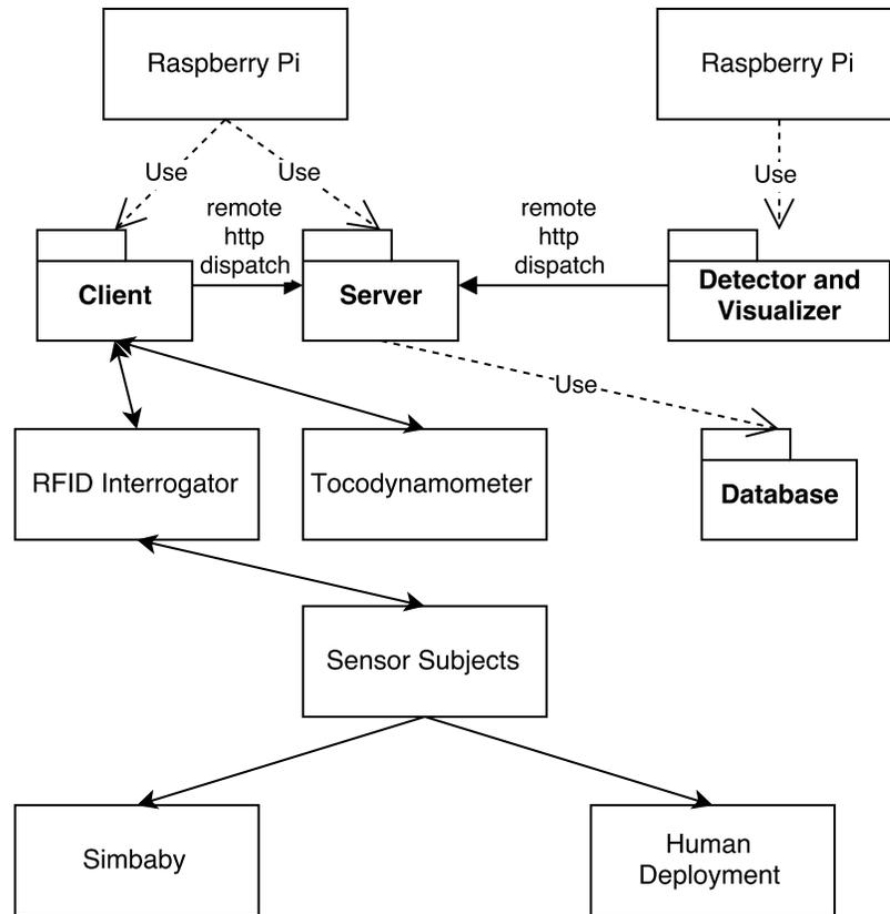
**Figure 4.3:** Communications diagram of the sensor data collection system that interfaces with the interrogator software described in Figure 4.8; here, a single entity or software class is depicted as a rectangle, a packaged collection of software classes is depicted as a folder, and arrows indicate that an entity invokes (“uses”) or communicates with (“http remote dispatch”) another entity
