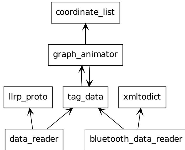
**Figure 4.5:** RFID UML Package Diagram
