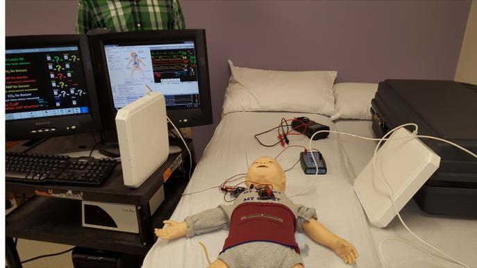
**Figure 13.1:** An example physical deployment according to Figure 4.3 in which the Bellyband is actuated by the SimBaby simulator while an RFID-based heart monitor is simultaneously interrogated by the client driver described in Figure 4.8
