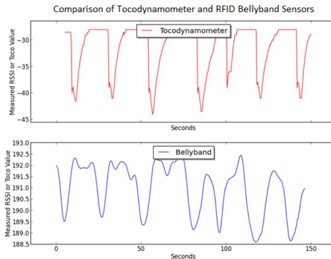
**Figure 11.3:** Tocodynamometer data collected from a programmable mannequin, at a range of approximately 3 feet (top), and Bellyband data simultaneously collected and filtered (bottom)
