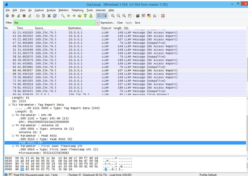
**Figure 2.4:** Capturing a set of Reader Operation (RO) RFID tag messages from the Impinj Speedway R420 interrogator
