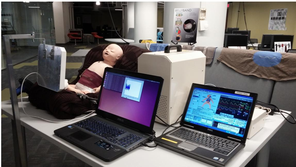
**Figure 11.2:** The SimBaby control software (right) configuring the automated respiratory patterns of the SimBaby mannequin (left), with RFID monitoring visualization depicted (center)
