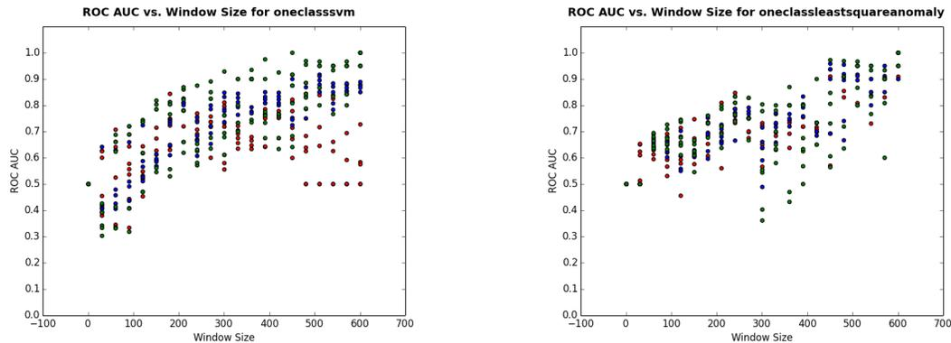
**Figure 6.5:** One-Class Support Vector Machine (left) and Least Square Anomaly Detector (right) executed over each specified configuration, and ROC AUC plotted against window size. Darker nodes, towards the upper portion of the plot, indicate larger training set sizes.
