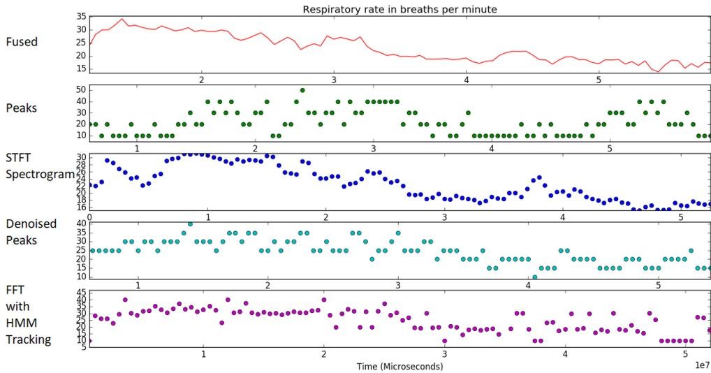
**Figure 9.1:** Results from the Expectation Maximization sensor fusion algorithm removing noise artifacts from individual measurement estimates
