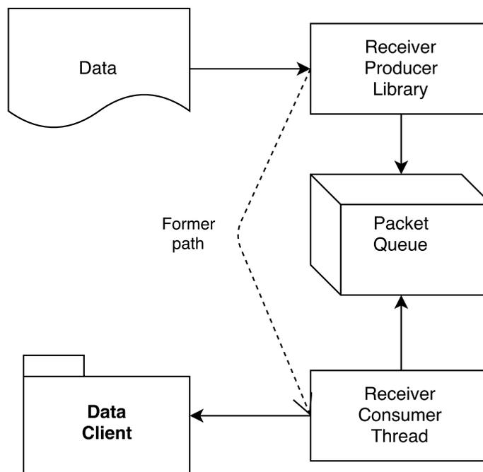
**Figure 4.14:** The classic Producer-Consumer threading model enables a producer thread to append data to a queue, where a consumer thread retrieves that data and performs deferred processing while the producer thread simultaneously obtains or generates more data to be processed
