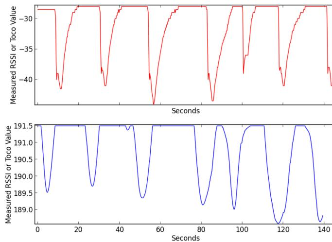
**Figure 4.2:** Visualization of data collected from a Tocodynamometer (top) and RFID (bottom), with a Gaussian filter and saturation point applied
