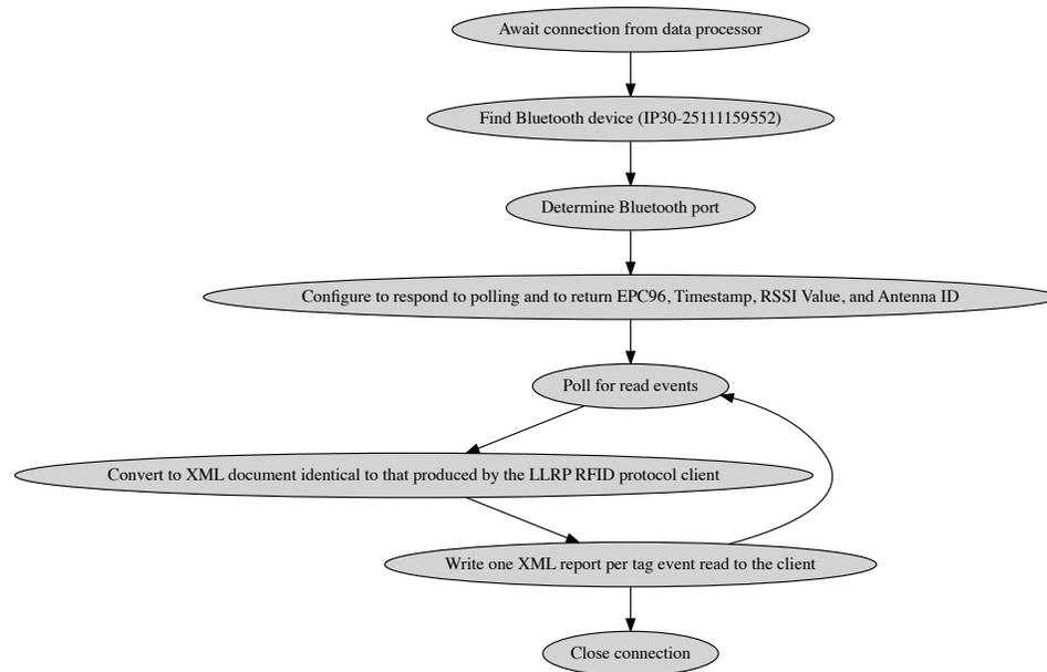
**Figure 4.11:** Bluetooth Portable RFID Server Module Custom Protocol Workflow
