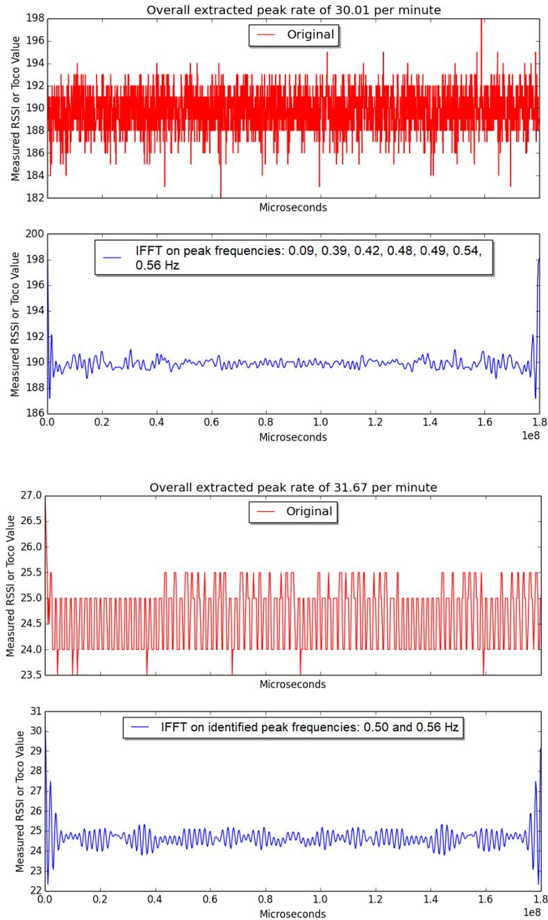
**Figure 7.1:** Bellyband data collected and filtered to estimate the target respiration frequency of 0.5 Hz (top), and tocodynamometer data simultaneously collected and filtered from the same mannequin, also estimating the same target respiration frequency of 0.5 Hz (bottom); the IFFT average yielded a predicted rate of 30.01 respirations per minute (top), as opposed to an estimated ground truth of 31.67 respirations per minute (bottom)
