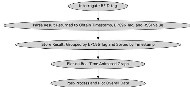
**Figure 2.1:** RFID Capture Workflow
