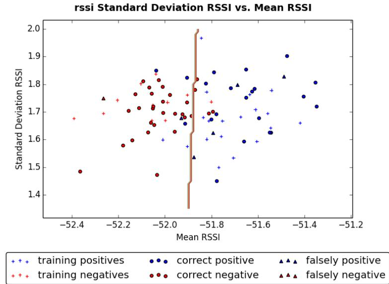
**Figure 5.1:** Bellyband data observed on a programmable mannequin, classified into actuating (blue) and non-actuating (red) classes: non-actuating training examples are generated using a subset of the actuating training examples, and the resulting Support Vector Machine classification performance on subsequent testing data is shown as circles (correct) and triangles (incorrect)
