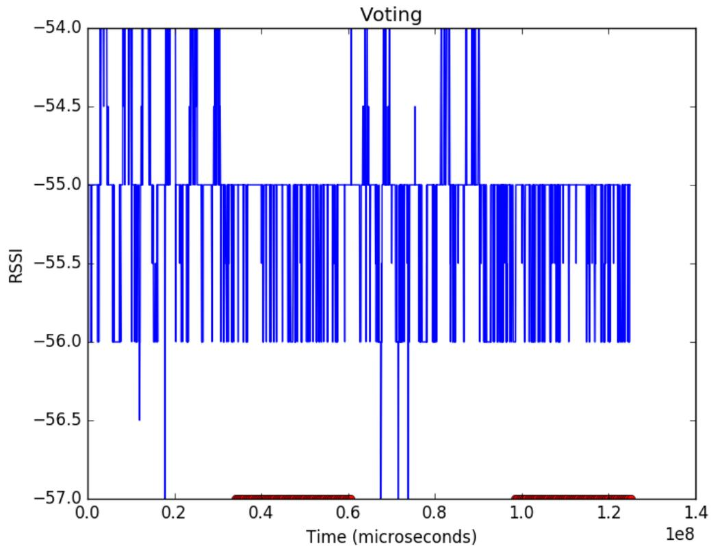
**Figure 12.8:** Classification using voting on multiple MCMC simulator measurements for a human trial at a varying respiratory rate with brief cessations: cessation periods are classified along the bottom of the plot
