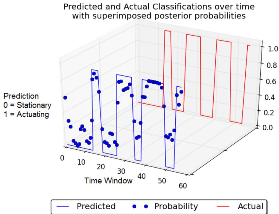
**Figure 12.5:** Predictive classification between breathing and non-breathing classes using the posterior probability trend with a programmable mannequin SimBaby alternating between breathing at an arbitrary rate and apnea (true class depicted in red); using probabilistic classification, changes in posterior probability are correctly classified before the linear perceptron alone would have
