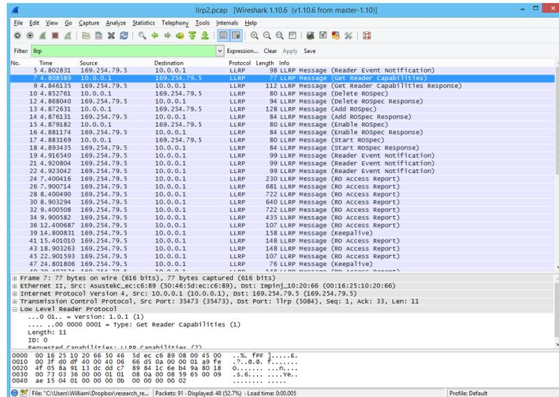
**Figure 2.3:** Opening an LLRP Session with the Impinj Speedway R420 interrogator, as captured by Wireshark. Notice the raw binary data to be parsed at the bottom of the figure, parsed by Wireshark for analysis.
