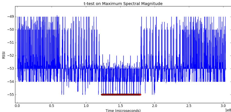
**Figure 6.6:** Using a t-test on a SimBaby mannequin programmed to cease respiratory activity from 120-180 seconds, breathing at a rate of 15 from 60-120 and 180-240 seconds, and breathing at a rate of 30 from 0-60 and 240-300 seconds; a 20 second training period was used, and detection of respiratory cessation is denoted in red
