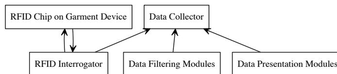
**Figure 2.2:** General system architecture for RFID interrogation
