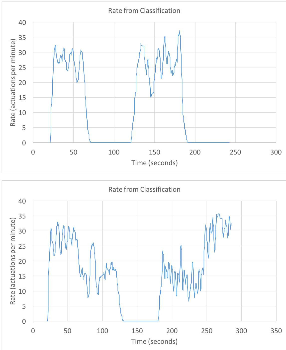
**Figure 12.9:** Rate estimation over time for two experimental runs (top: stretching at 31, 0, 31, 0 per minute for 1 minute each, and bottom: stretching at 31, 15, 0, 15, 31 per minute for 1 minute each), computed as the number of actuation classifications made in the past  $k = 6$  seconds extrapolated to a one-minute rate. Note that the plots begin after 20 seconds because the first 20 seconds of data are reserved for training the classifier used in computing the rates.
