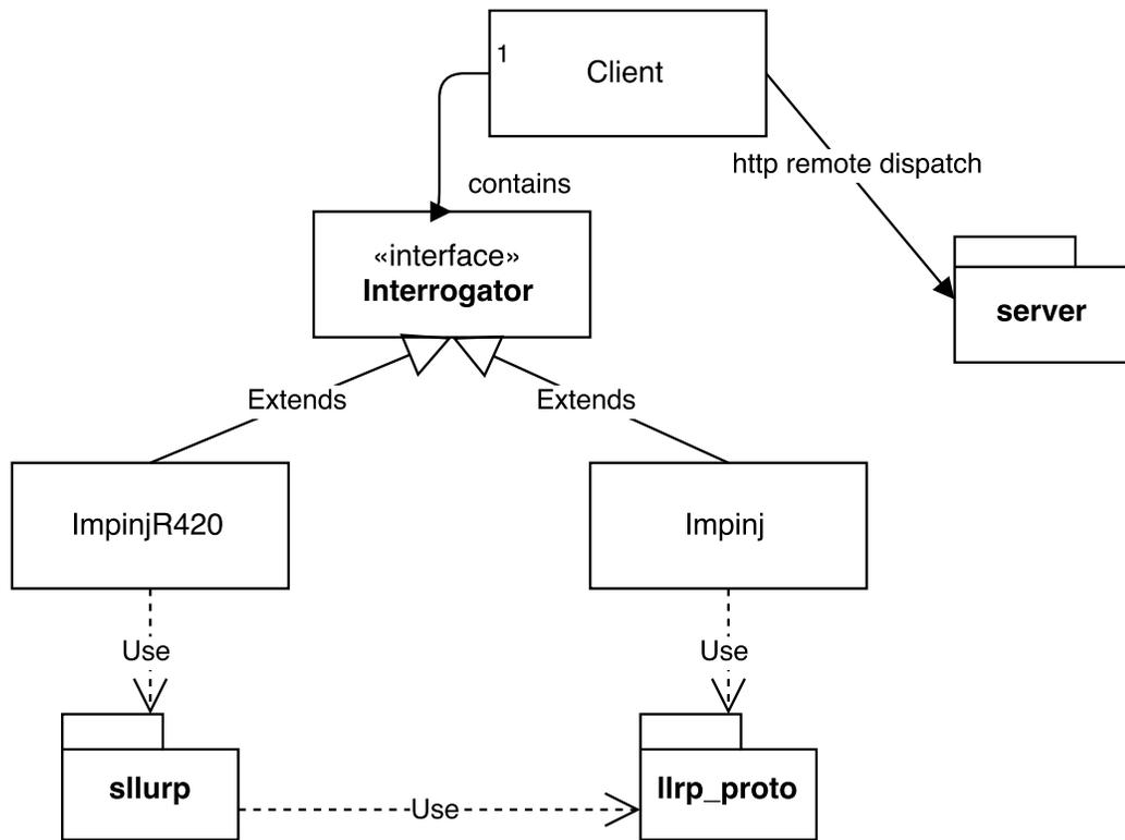
**Figure 4.8:** High level design of software interface to drive the RFID interrogator, storing time-series data captured into the backend database via HTTP web service calls to the web service depicted in Figure 4.9
