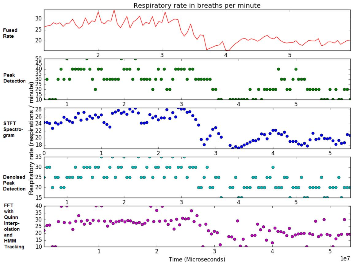
**Figure 12.10:** Individual observed measures and their fusion over time for a human subject breathing at a rate of approximately 30 for 30 seconds, and at a rate of approximately 15 for 30 seconds
